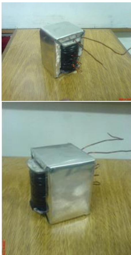
Figure 10 Photos of the transformer designed and built, ready to be attached to the handle of the pyrograph
