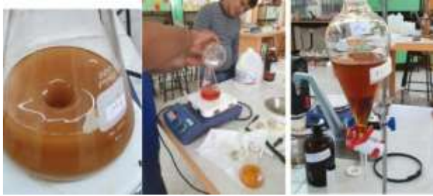
Figure 5. A) Esterification process, b) transesterification process to obtain biodiesel and the by-product glycerine Own Source
