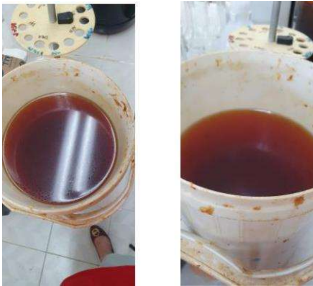
Figure 6 Glycerin obtained from the production of biodiesel in the Institute's chemistry laboratory Own Source
