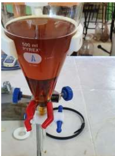
Figure 2 Transesterification process to obtain biodiesel and dark brown glycerin, Own Source
