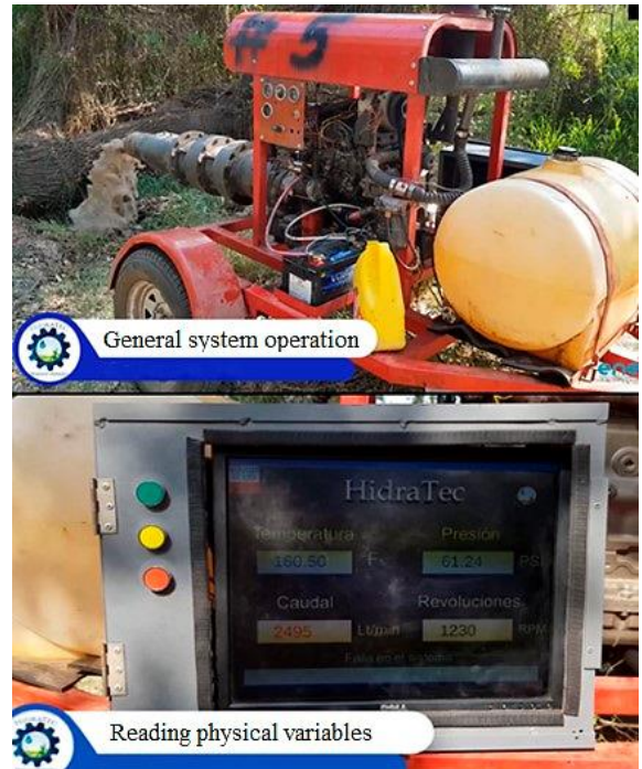
Figure 13 Monitoring system in field tests Source: Own elaboration with tests carried out (2019)
