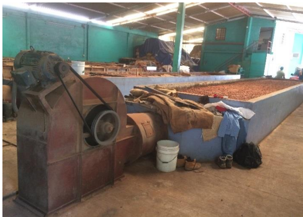
Figure 3 Samoa type dryer Source: Own photo
