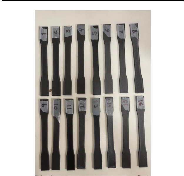
Figure 8 ASTM D638 models printed on FFF with PETG-CF according to DOE orthogonal array L 16
