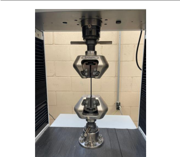
Figure 9 Tensioning machine performing tensile work on specimen
