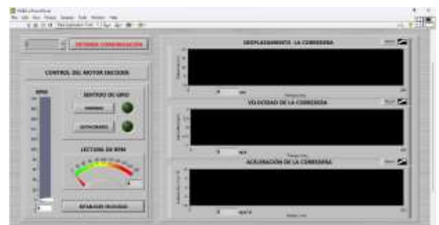
Figure 12 Control and monitoring panel in LabVIEW Source: Own Source
