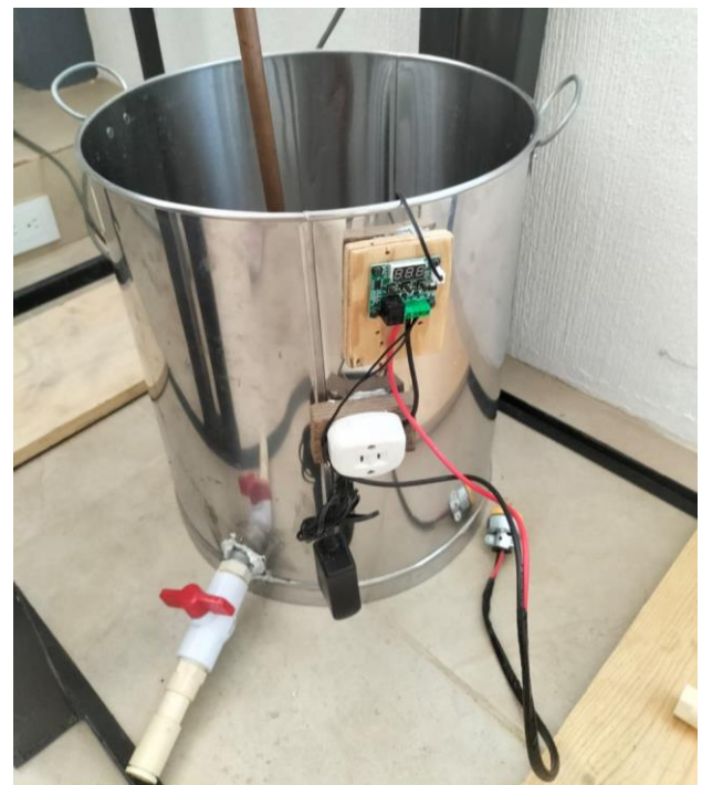
Figure 3 Macerator with temperature control, showing the display on the outside of the prototype
