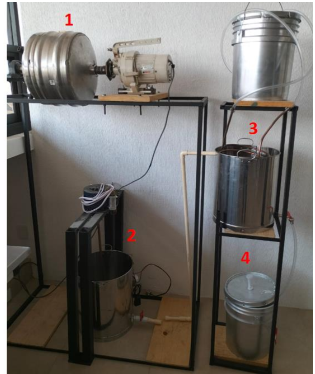
Figure 6 Unit operation system consisting of: 1: mill, 2: macerator, 3: cooler, and 4: fermenter
