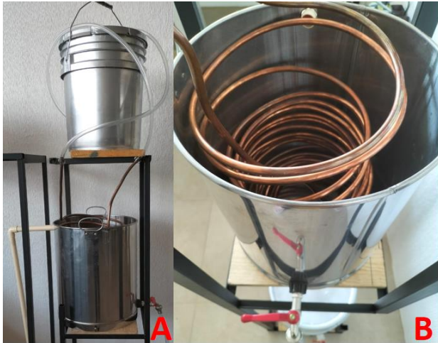
Figure 4 Cooler prototype. A: external view of the cooler. B: view of the copper coil inside the cooler
