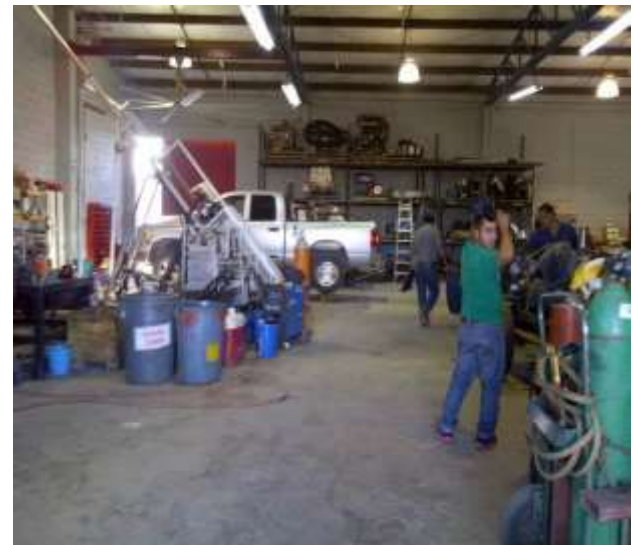
Figure 1 Accumulation of material and undefined areas in the workshop
