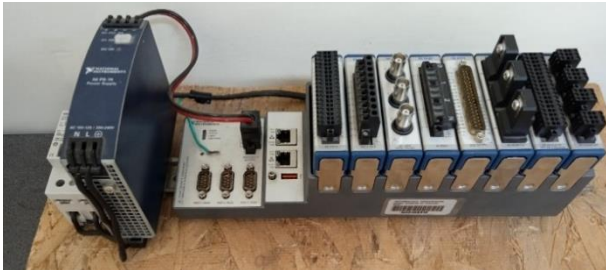
Figure 3 CompactRIO-9068 Data Acquisition (DAQ) System
