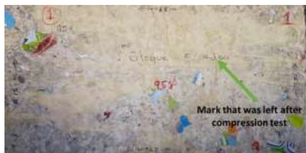
Figure 5 Appearance of the agglomerate after subjecting it to the compression test Source: Own Elaboration
