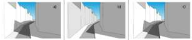
Figure 8 Section 4 (S4), shadow projection in (a) March, (b) June and (c) September
