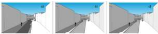
Figure 6. Section 2 (S2), the shadow projection in a) March, b) June, c) September
